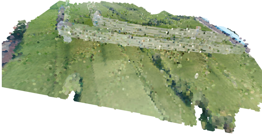
Figure 3.2. Voxel grid (voxel-size = 0.03)
